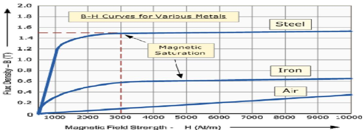
Figure 3: B-H Curve for magnetic materials
